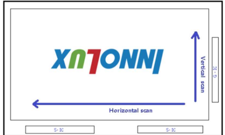
Fig. 1 Normal scan (Pin24, Reverse = Low or NC) Fig. 2 Reverse scan (Pin24, Reverse = High)
